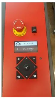
Use the arrow keys to navigate to the z-axis setting
