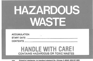
When the container is placed in the appropriate Waste Storage Area designated for your laboratory the Hazardous Waste label must be put over the USED CHEMICAL LABEL name and date it:
