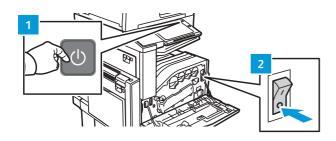
To restart the printer, on the control panel, press the **secondary power switch**.
