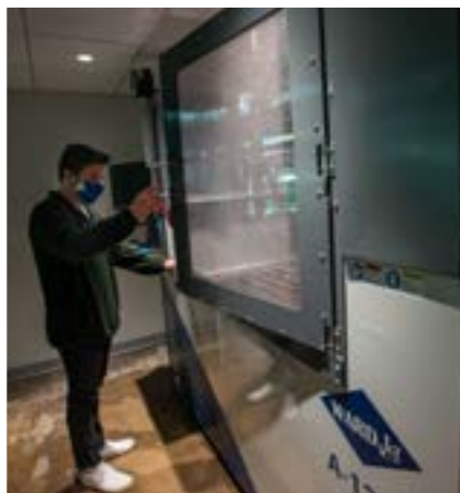
DI Crew student employee Foster Rak at the waterjet cutter in the Waterjet Shop of the DI Reactor on the lower floor of the new DI Hub. A waterjet cutter can cut through any known material—making it one of the most versatile machines available.
